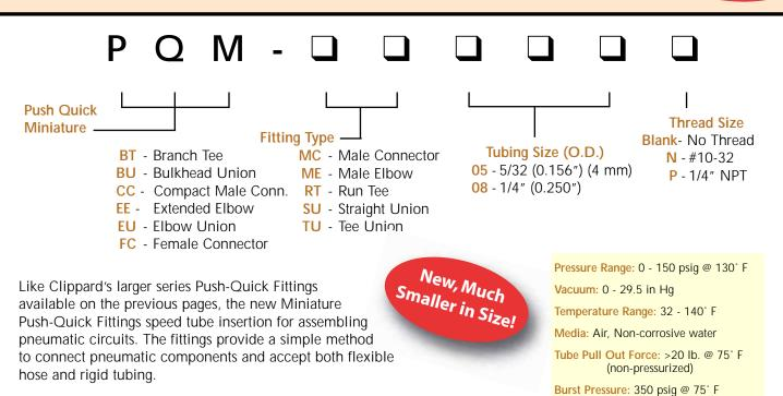
Available in 5/32" (4 mm) and 1/4" OD tubing, the fittings permit full flow through the ID and there is no small orifice as required with barb fittings. They are available in many configurations with preapplied thread sealant.
